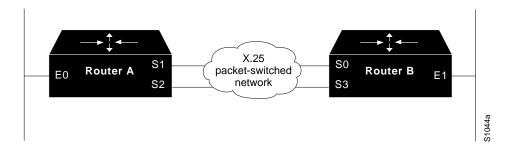
**Note** All four serial ports configured for the two routers in the following configuration example must be assigned to the same IP subnet address space. In this case, the subnet is 131.108.170.0.
