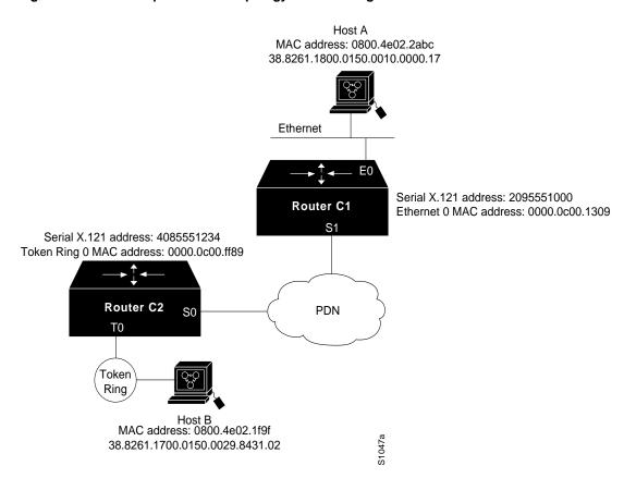
Figure 13-7 **Example Network Topology for Switching CMNS over a PDN**
