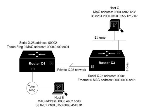
A key difference for this configuration compared with the previous example is that with no PDN, the specification of an X.121 address in the **x25 map cmns** command is not necessary. The specification of an X.25 address also is not needed, but is included for symmetry with the previous example.
