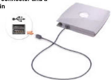
D/Bay connector includes a USB 2.0 connector and a power pin
