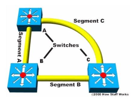
Even if one of the switches fails, the network continues. This setup provides redundancy and effectively eliminates the single point of failure.
