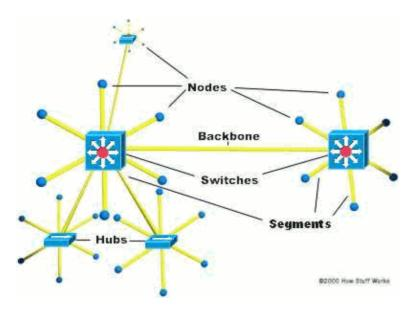
Most networks are not fully switched because replacement of all the hubs with switches is costly. Instead, a combination of switches and hubs create an efficient yet cost–effective network. For example, a company can have hubs that connect the computers in each department and a switch that connects all the department–level hubs together.
