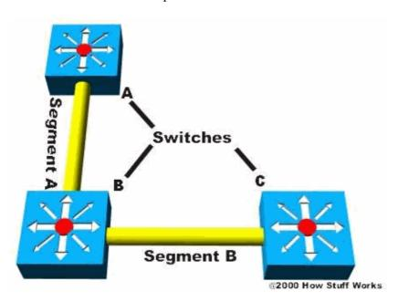
If either switch A or C fails, the failure affects the nodes that connect to that switch. But nodes at the other two switches can still communicate. If switch B fails, the failure brings down the entire network. What if you add another segment that connects switches A and C?
